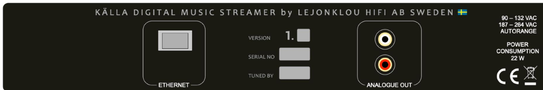
**Start** by connecting an Ethernet cable between the router of your local network and Källa. Make sure **there isn't excessive strain** on Källa's Ethernet port. It's often beneficial to have a network switch (e.g. Netgear GS-108T) in between the router and Källa. We recommend that the Ethernet cables are kept as short as possible, but never shorter than 2.5 m.
